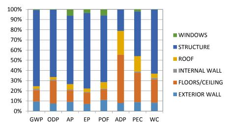
Figure 3.8. Contribution of building elements to the production stage environmental impacts of 1m<sup>2</sup> of a hypothetical office building located in London Source: JRC-IPTS (2011)
